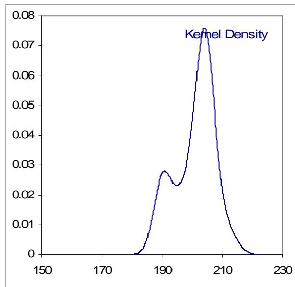
Determination of Kinematic Viscosity @ 40°C on sample #11042; results in mm<sup>2</sup>/s
