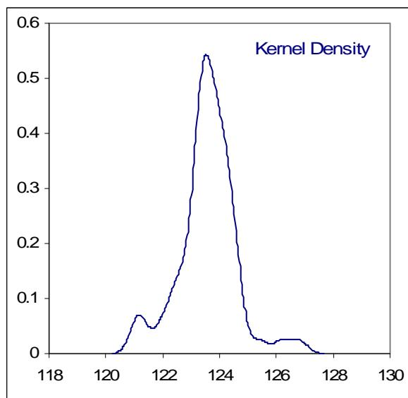
Determination of Kinematic Viscosity @ 100°C on sample #11042; results in mm<sup>2</sup>/s
